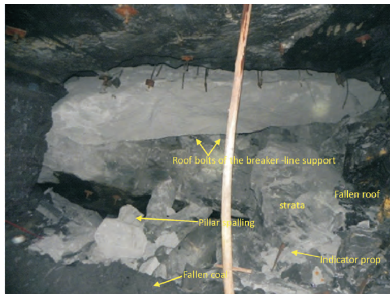
Roof bolt based breaker line failure related goaf encroachment during caving of the roof strata.
