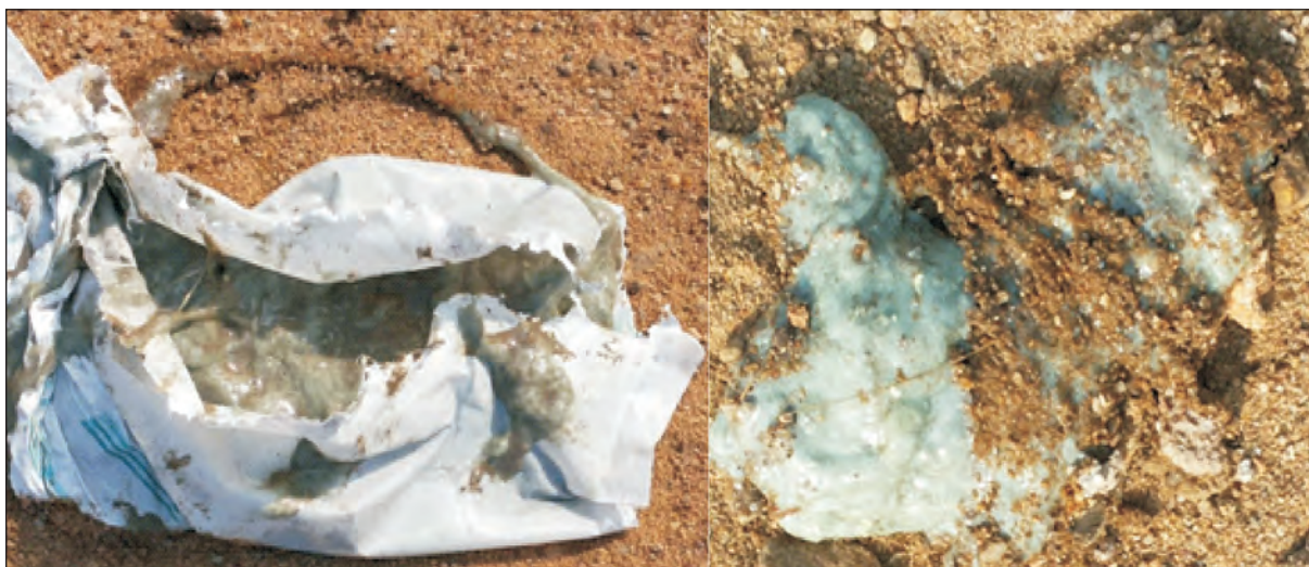
Figure 1: Photographs Of Scattered Pieces Of Misfired Ld Column Explosive Salvo Power (Batch No.- 4060, Dom :- 31.12.2015) Of M/S Salvo Explosives & Chemicals Pvt. Ltd., Secunderabad
