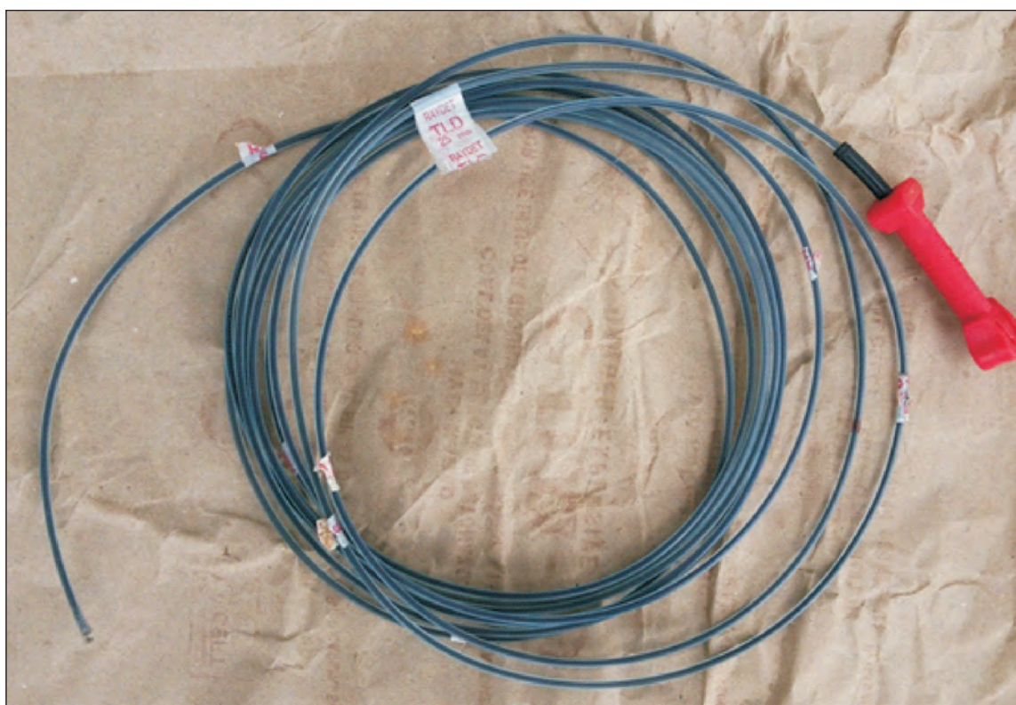
Figure 2: Photograph Of Misfired Nonel Of M/S Goel (Raydet, Tld, 25Ms, Batch / Case No. - 63 & Date Of Manufacture - 02.06.2015)
